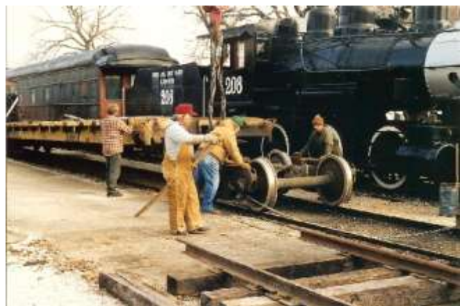
A crane lifted the flat car so one truck could be removed. The locomotive in the background might be owned by Fort Worth-based Trinity Valley.
