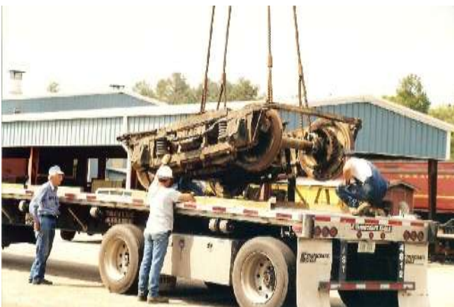
Trucks and other components were loaded onto a flatbed truck bound for Fort Worth. Blair Lavell, shop superintendent for the TSRR, watched as items were dismantled and loaded for shipment.
