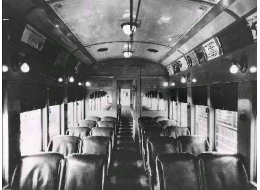
Interior of motorcar showing painted mahogany, blue and white linoleum, and newly installed side wall sconces. Original bench seats replaced by double bucket style seat.
